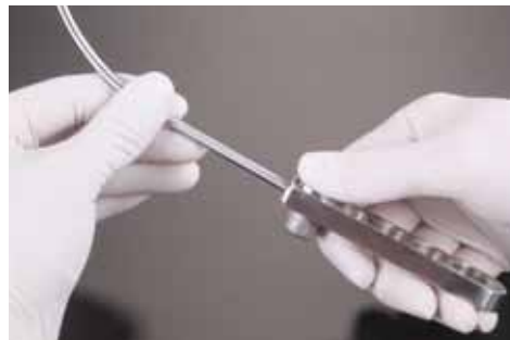
4. Press the locking element down
